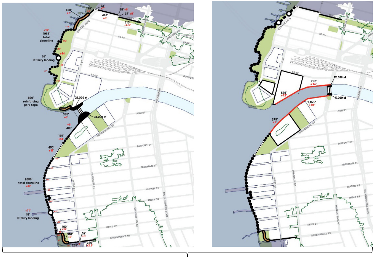
FIGURE 9-1 Barrier options, Newtown Creek: Left: 2nd Street Alignment (Barrier II); Right: Manhattan Avenue Alignment (Barrier I)
