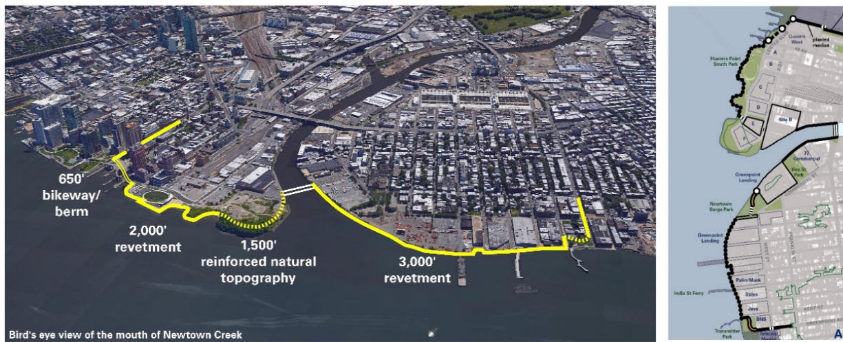
FIGURE ES-7 Preferred Concept Options: Shoreline Alignment with 2nd Street or Manhattan Ave In-water Barrier
